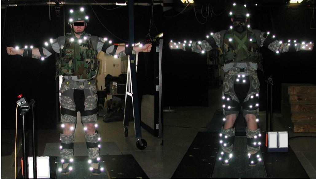
Figure 5. Front and rear views of test volunteer in full extremity armor condition with passive reflective motion capture markers for the static calibration capture. Tracking markers for the body segments as well as joint markers are worn in this picture. After the static calibration capture, joint markers at the ankles, knees, elbows, and wrists are removed.
