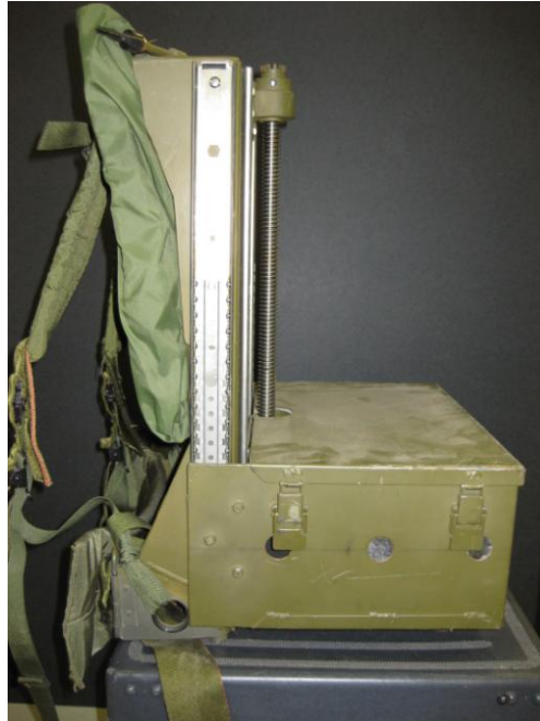
Figure 3. Experimental military backpack for load carriage research. The customized “ALICE” backpack was designed specifically for laboratory testing of the effects of center of mass (COM) position on gait and metabolic cost. This prototype allowed for quick adjustment of the COM of the load by cranking the lead block containing load compartment up and down the frame of the pack.
